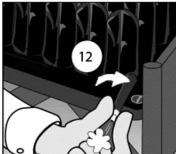
12. Turn valve to close. (Repeat steps 9 - 12 for remaining air valves on multi-valve cushions.)
